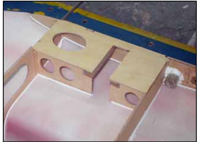
The plywood landing gear mount is now even stronger than the original Rookie, and is aligned with a jig in the mould before joining.
