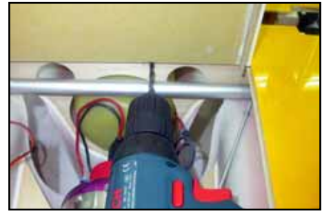
(above) Drill a 8mm Ø hole thru' the rear bulkhead for the thrust vector linkage as shown.
