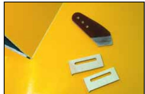
(above/below) Prepare the bottom of the phenolic horn as shown, and glue into the 2 slotted plywood parts securely.
